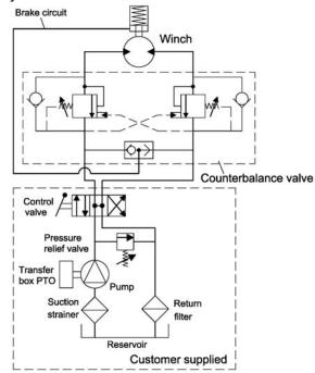
( Powered by PTO / power take off unit driven pump )
