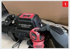
Powering off the winch receiver module and the wireless transmitter
