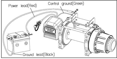
▶ Nut fastening for motor & contactor
